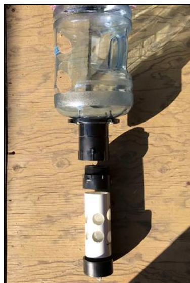
Figure 5. Main body of trap with foam float attached and cod end pieces staged for assembly.
