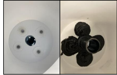
Figure 6. Left: Inside bottom of bucket with bolts and plastic washers. Right: 4" PVC or ABS coupling caulked in place along with bolts and washers.
