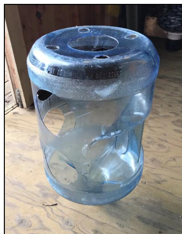
Figure 4. Main body of trap with 7 – 4” holes drilled in the side and top for funnels and lighting unit installation.
