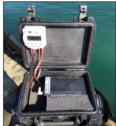
Figure 10. Light unit configuration with 12V lithium-ion battery and programmable timer.
