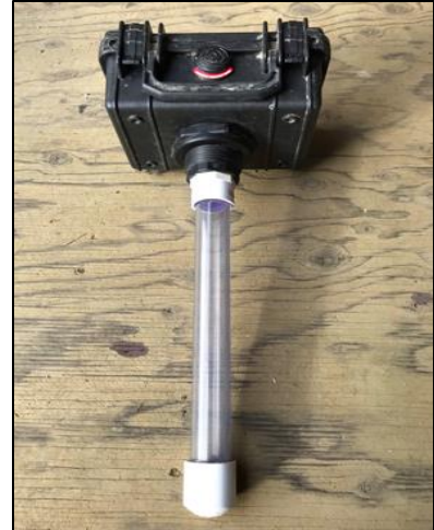
Figure 9. Light housing consisting of Pelican box, bulkhead fitting, and capped PVC pipe.
