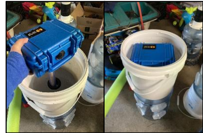
Figure 7. Left: Bucket top with coupling and foam rounds installed. Right: Fully assembled bucket top with Pelican case.
